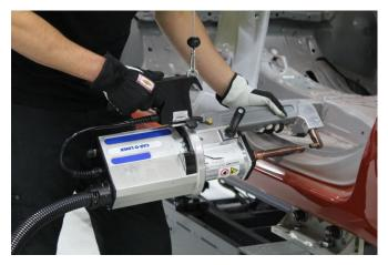
A wide variety of yokes allows for accurate spot welds anywhere around the vehicle.
